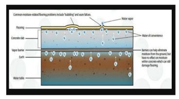
HydroBlok Primer 1100 is an impermeable two-component modified epoxy coating with zero VOC to block the moisture vapor emissions from new and existing concrete slabs. Its unsurpassed adhesion to concrete exceeding 1,100 psi tenaciously grabs onto the concrete slab to block the moisture and vapors beneath the concrete slab. For extra protection, we recommend applying HydroBlok Polyaspartic topcoat.
